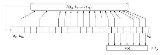
Figure 3: Linear feedforward function for NLFSR A
