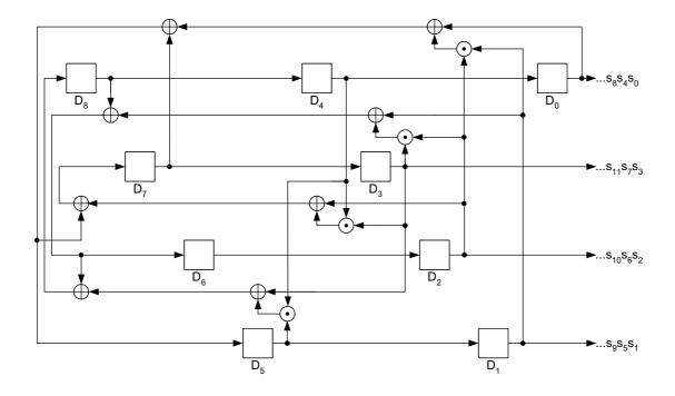
The next figure shows the implementation of the FSR for step size k = 4.
