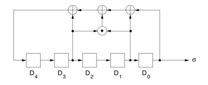
Figure 5: A primitive 5-stage NLFSR
