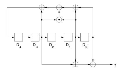
Figure 6: The 5-stage NLFSR with linear feedforward output function
