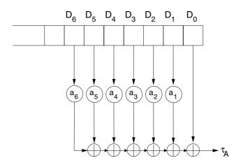
Figure 4: Linear feedforward function for NLFSR A: enlarged
